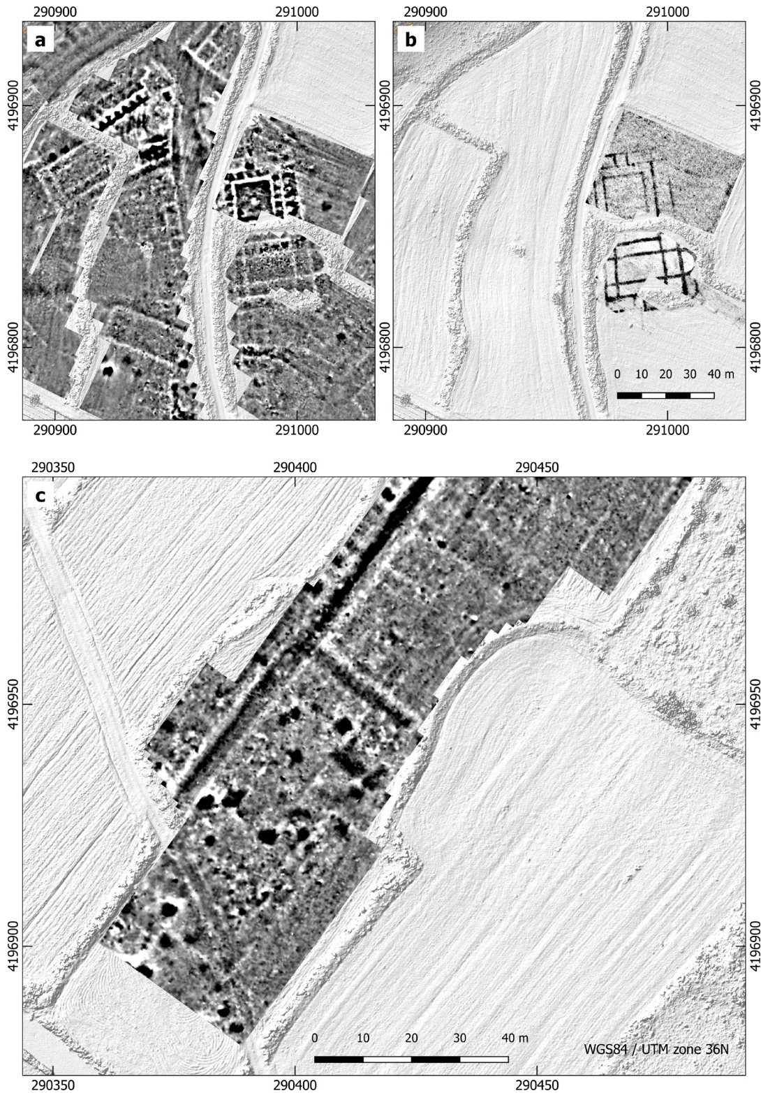
Fig. 3: a) this part of the magnetic map indicates the central public area (-20/+20 nT, white to black); b) in the radar measurement, the Macellum and the Basilica are partly more clearly visible than in the magnetogram; c) assumed center of brick or pottery production in area 592 and 608.
